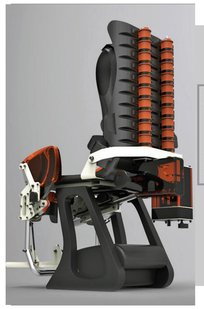
SACE 2 is a robot, an exoskeleton, connected to the human Body it can restrict or help the movements. Even the artificial spine can flex through a cable system
